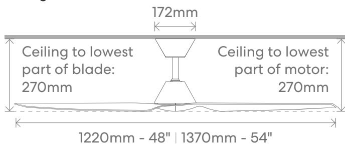
Dimensions based off supplied 600mm Rod
