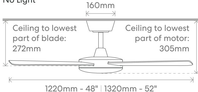
Dimensions based off supplied 139mm Rod
