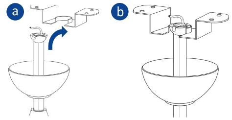
iii. Align ball groove on hanging ball with ridge on hanging bracket.
