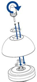
4. Align the blades with screw holes on motor housing, and secure with the screws and the blade fixing plate.
