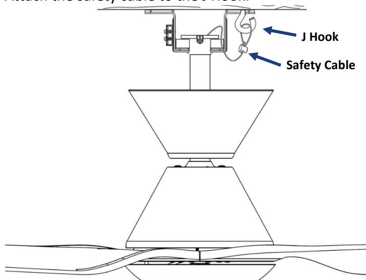
11. Place receiver in the hanging bracket and follow the wire diagram to connect wires and connectors. Ensure cables are neat and tidy. Connect power, receiver and the fan as per electrical wiring diagram.
