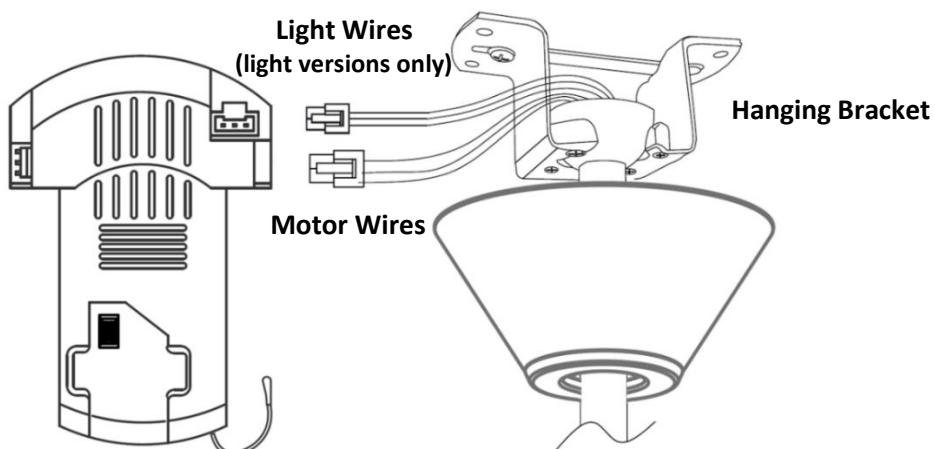
12. Push the canopy towards the ceiling to cover the mounting bracket, receiver and wires.
