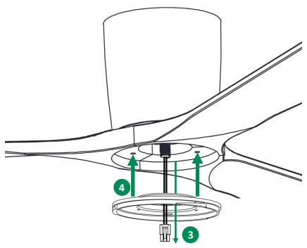
4. Connect the push plug wire of the Light Kit to the push plug wire from the motor.
