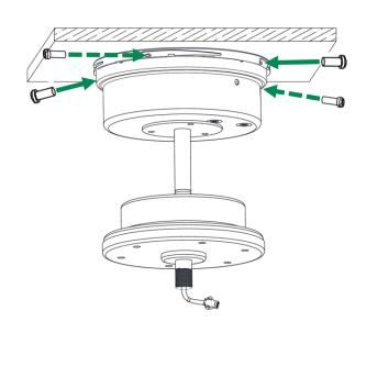
8. Slide the motor housing up to the motor assembly.
