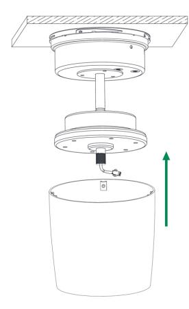
9. Align the grooves of the motor housing to the grooves of the hanging plate and twist into place.
