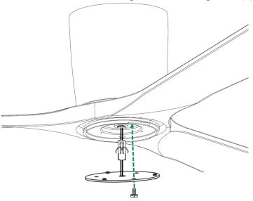
7. Align the grooves of the Light Ring with the grooves of the Light Kit Plate and twist into place.
