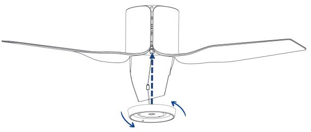
4. Fix into place with three (3) screws and tighten.
