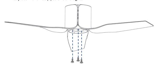
5. Align the grooves of the Diffuser with the grooves Light Kit and twist into place.
