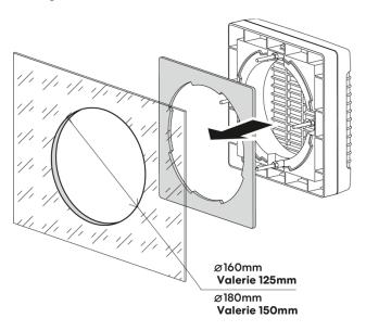
**STEP 6** – Insert the second sealing gasket onto the other side of the glass. Use the bolts as guides to get them onto the internal intermediary casing. Avoid the sealing gasket from jamming. Fasten the casing tightly by means of threading the plastic nuts on the bolt ends and tighten them in turn.
