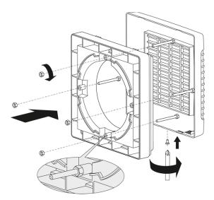
**STEP 5** – The fan is designed for mounting on glass (partition) with 4 to 17 mm thickness. To install the fan with the impeller diameter 125 mm cut  $\emptyset$ 160 mm hole in the glass and for the fan with the impeller diameter 150 mm cut  $\emptyset$  180 mm hole. Insert one sealing gasket onto the pre-mounted casing and insert the unit into the cut-out hole.
