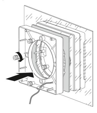
**STEP 7** – Thread the wire through the sleeve in the internal casing and though the hole in the main casing. If the casing does not feature a cut-out hole, then it must be cut out at this time. Fasten the main casing with the 4 included screws.
