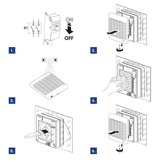
The product surfaces must be regularly cleaned from dirt and dust. Cut off power supply prior to any maintenance operations (See Step 1). Remove the front cover (Step 2), clean the fan following Step 3 and 4 using detergent and water to clean the external fan surfaces. To clean the internal fan surfaces, use a brush (Step 5). Mount the fan cover back on (Step 6) and connect the fan to power supply. For cleaning use a soft cloth or brush and mild detergent water solution.
