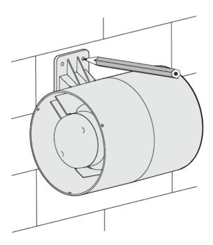
**STEP 4** – Drill the holes for the in compliance with the mounting seats on the fan casing and install the fan with screws. The power cable must be routed through the screwed cable gland. If required insert wall plugs into masonry if installing fan directly onto a brick wall.
