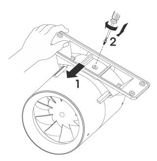
**STEP 3** - Position the fan in your preferred installation location and mark the position of the holes on the fan where the screws will then be placed.
