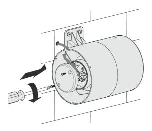
**STEP 8** – Connect ducting / pipe work of a matching diameter to fan as required.
