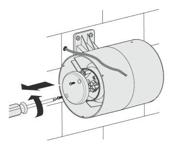
**STEP 6** – Connect the wire to the terminal box by following the wiring diagram. Install the retaining clamp back and secure it with the included screws.
